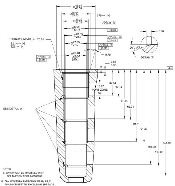
3.) IT IS VERY IMPORTANT THAT VALVE CAVITIES MEET ALL DIMENSIONAL AND QUALITY STANDARDS OF CONCENTRICITY AND PERPENDICULARITY. THREADS MUST BEPERPENDICULAR TO THE SPOTFACE SURFACE. SPOTFACE MUST CLEAN UP TO FULL DIAMETER. IMPROPERLY MACHINED CAVITIES CAN LEAD TO CARTRIDGE MALFUNCTION AND/OR FAILURE FROM DISTORTION.
