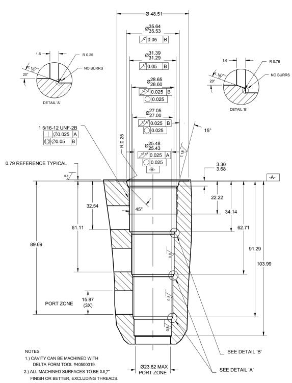
3.) IT IS VERY IMPORTANT THAT VALVE CAVITIES MEET ALL DIMENSIONAL AND QUALITY STANDARDS OF CONCENTRICITY AND PERPENDICULARITY. THREADS MUST BE PERPENDICULAR TO THE SPOTFACE SURFACE. SPOTFACE MUST CLEAN UP TO FULL DIAMETER. IMPROPERLY MACHINED CAVITIES CAN LEAD TO CARTRIDGE MALFUNCTION AND/OR FAILURE FROM DISTORTION.
