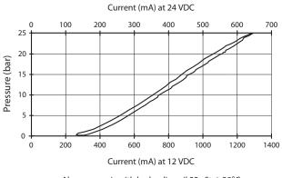
Above curve is with hydrauliuc oil 32 cSt @  $38^{\circ}C$
