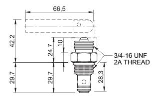
NOTE: (Ø11.1) cavity predrill depth must be 33.3 minimum from spotface.
