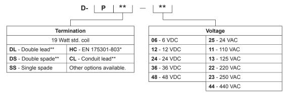
\*Formerly DIN 43650 Hirschmann connector. \*\*Only these coil terminations are stock.
